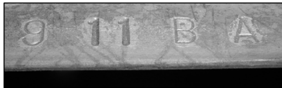
Figure 8. Address code for steel structure members. A manufacturer/installer of steel structures uses this code to tell laborers the location and orientation of the steel members (image courtesy of ConXtech).
