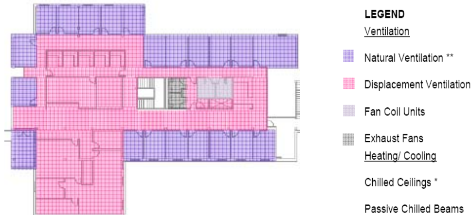
Figure 2: Mechanical zone plans did not convince the owners that this layout was correct. The zone plans were not consistent with other documentation, which made it difficult for other disciplines to coordinate with the mechanical engineers.
