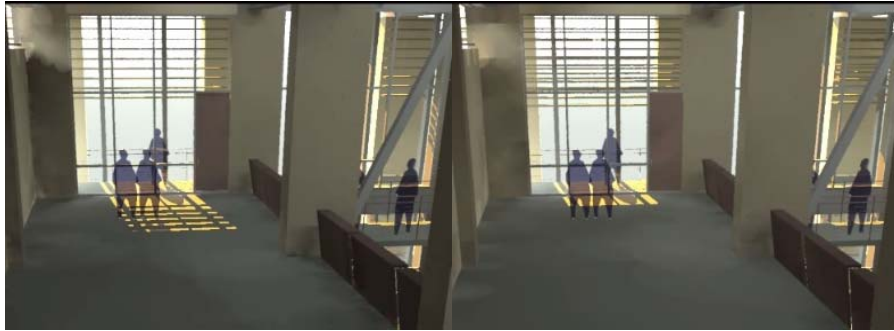
Figure 3. Snapshot of a QuickTime video. The consultants use this video to show the architects how different louver configurations affect daylighting in the GSB.
