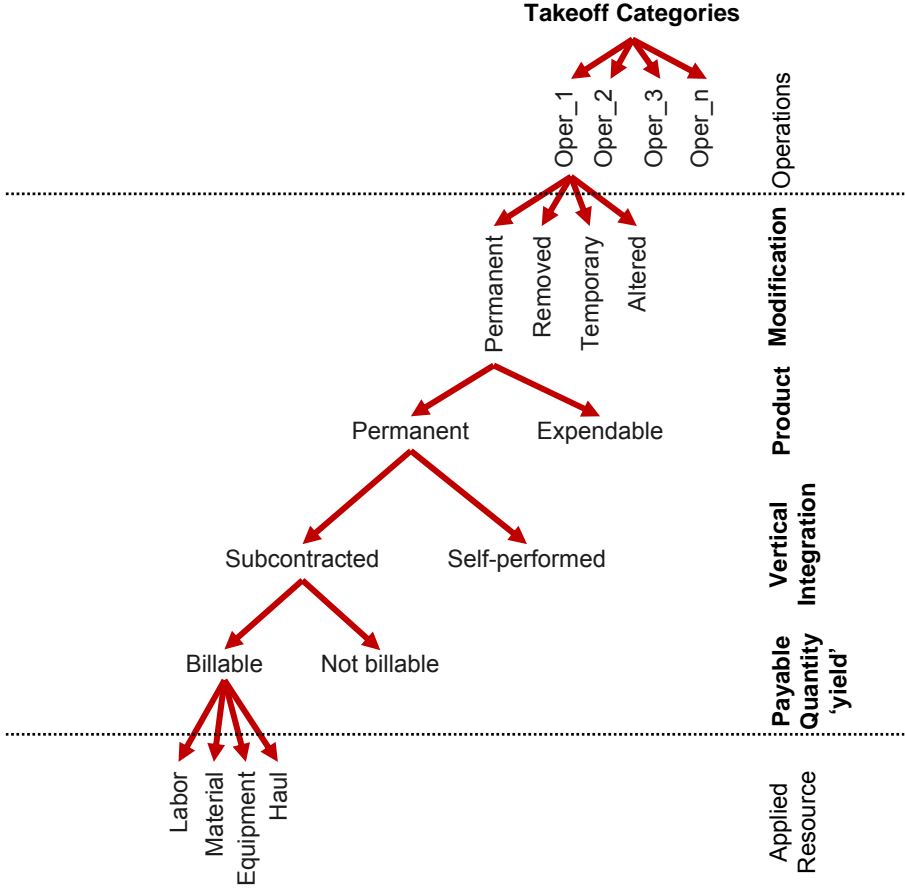
Figure 22 Bartholomew’s cost estimating breakdown structure; this breakdown structure is a suitable for suffix details in a chart of accounts. The bold categories are unique to Bartholomew’s breakdown. Some pragmatic breakdown structures I have seen used by civil contractors places the subcontractor as an applied resource – though as Bartholomew points out this prevents maintaining a parallel plan for use to audit the subcontractor.
