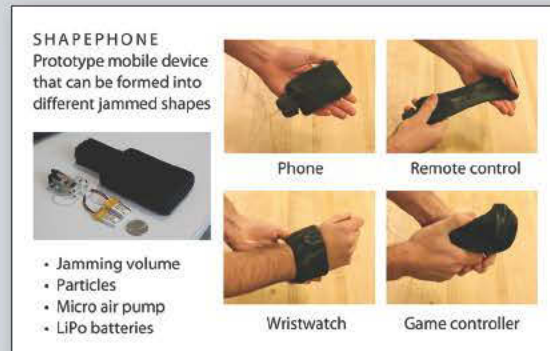
Figure 3. Shape-changing devices, such as Shapephone, can lock into different shapes using particle jamming.
