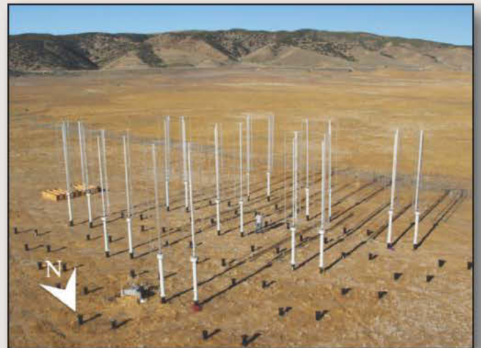
Field test of an array of vertical-axis wind turbines in southern California. Scale is indicated by the author, standing in the center of the array.
