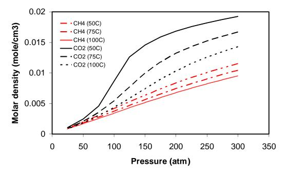
Figure 1: Molar density of CH<sub>4</sub> and CO<sub>2</sub>.
