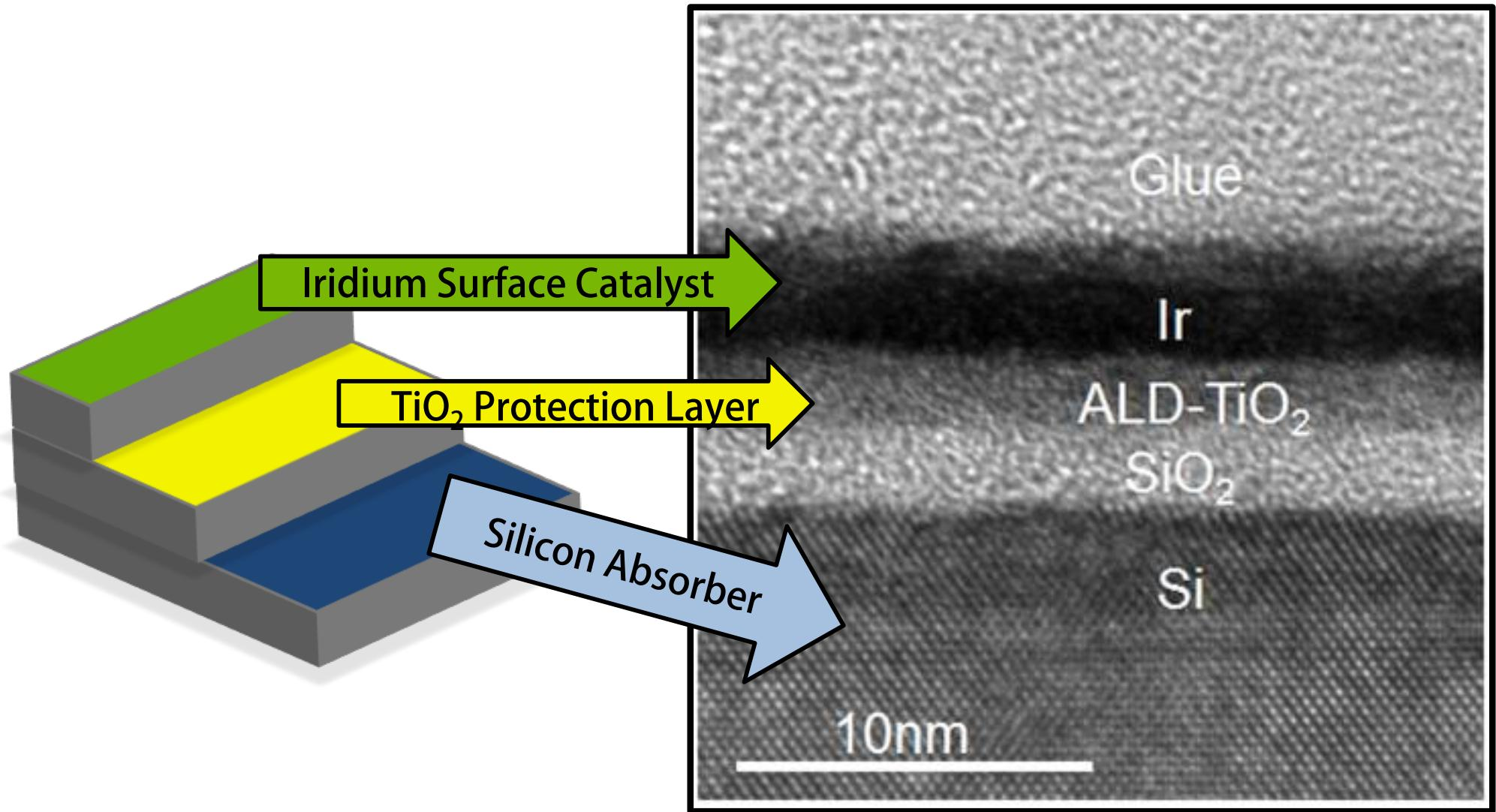
*ALD-TiO<sub>2</sub> Tunnel Oxide on Silicon
