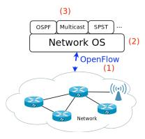
Figure 1: Components of SDN
