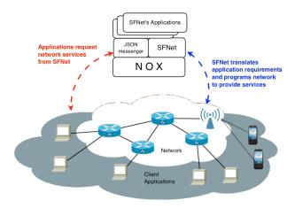
Figure 2: Architecture of SFNet
