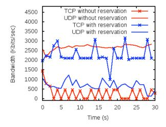
Figure 5: Available TCP bandwidth with(out) SFNet's reservation
