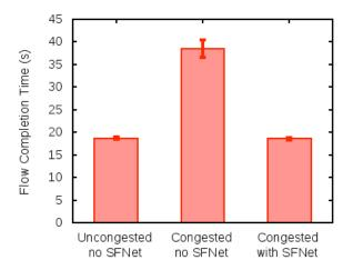
Figure 4: Flow completion time with(out) SFNet's congestion enquiry
