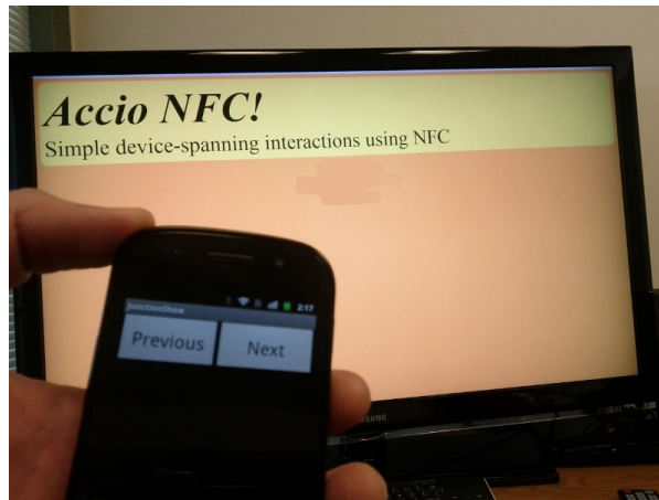
Fig. 3. A PocketSlides slideshow run between a phone and a display.
