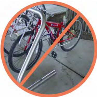
Figure D-4: “Coat-hanger” rack (not recommended)
