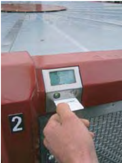
Figure D-11: Electronic locker smart card reader
