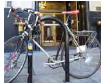
Figure D-1: Inverted U- rack (recommended)
