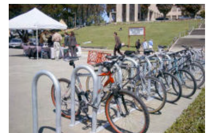
Figure D-2: Multiple inverted U- racks (recommended)
