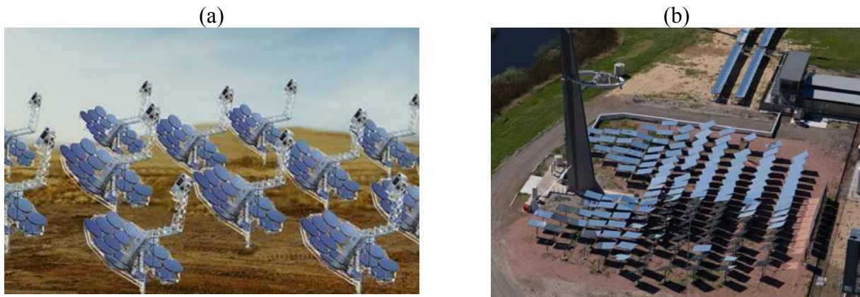
5 Figure 3.16: (a) Rendering of aggregated dish/Stirling units, and (b) a sister tower of one to be 6 used for powering a Brayton cycle microturbine (courtesy CSIRO).
