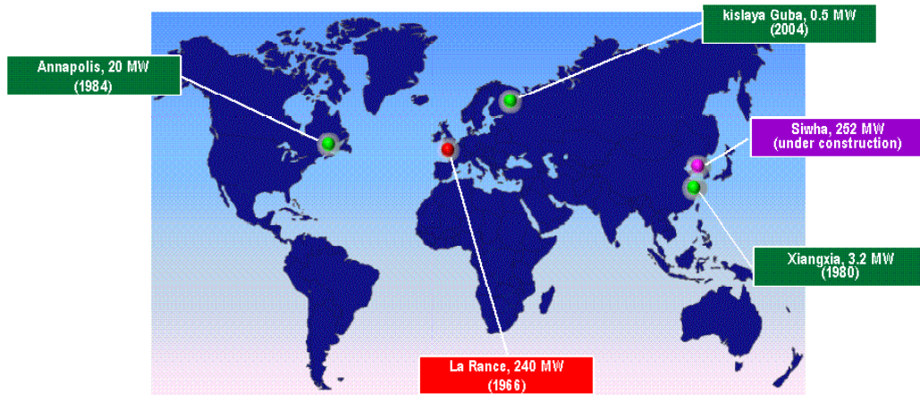
3 4 Figure 6.22: Tidal rise and fall power station in operation as of March 2009 (courtesy EDF) [TSU: 5 status of source?]
