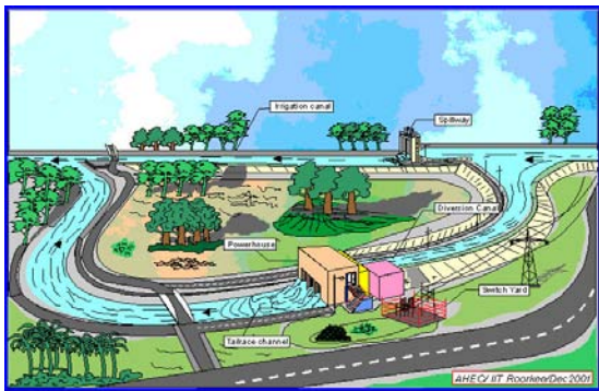
Figure 5.9: Typical arrangement of instream technology hydropower projects.
