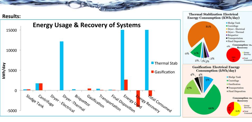
**Conclusion:** Gasification possesses a significant energy recovery system and also significantly reduces the overall energy requirements when compared to Thermal Stabilization. Further work in final deposition is still needed, but it is hypothesized that Thermal Stabilization will have an approximate 20 to 40 % energy recovery while Gasification will still remain as the optimum sludge treatment technology with 61% energy recovery.
