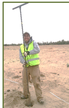
Drilling CZ borehole
