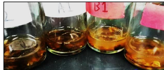
Sterile (left) and non-sterile (right) woodchip & stormwater media after seven days of fungus incubation.
