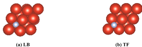
Figure 5. Optimized structures of atomic nitrogen adsorption at 0.25 ML surface coverage on (a) LB and (b) TF sites.
