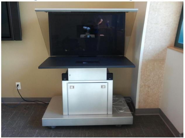
The TelePresence unit is a standard videoconferencing unit using H.323 protocol, so should be able to communicate through an internet (IP) connection to any other standard H.323 videoconferencing unit. The device is particular in the use of the image-splitting glass reflector, which allows you to look at the other party at eye level.
