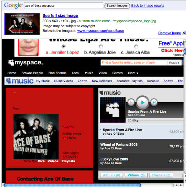
Figure 6: Because MySpace whitelists Google in the document referrer, an attacker’s site can use Google Image search to launch clickjacking attacks on MySpace.
