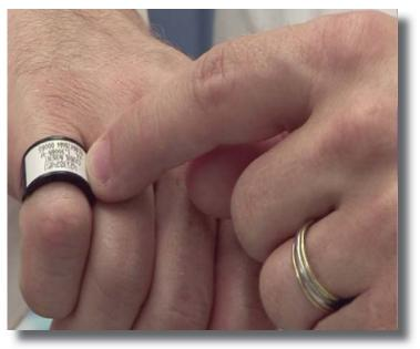
Finger-ring dosimeters are used by some radiation workers to monitor radiation exposure.
