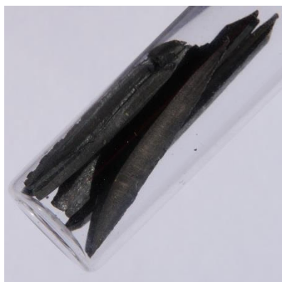
Pieces of lithium with visible lithium nitride tarnish.
