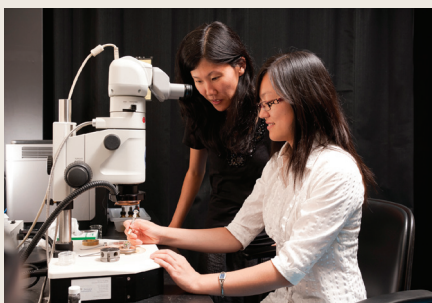
Graduate student Yu Lin loads glassy carbon spheres into a sample chamber where they will be compressed by a pair of diamond anvils. Wendy Mao, assistant professor of Geological and Environmental Sciences, looks on.
