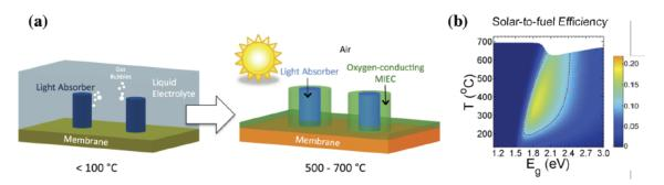
Figure 1: (a) Schematic comparison of the liquid-based PEC operating at room temperature versus the proposed solid-state (photo-anode) PEC operating at elevated temperature. (b) Simulated solar-to-fuel efficiency of the proposed PEC design. The white region indicates temperatures that are unreachable due to insufficient solar energy input. The dotted line indicates a 10% efficiency boundary.
