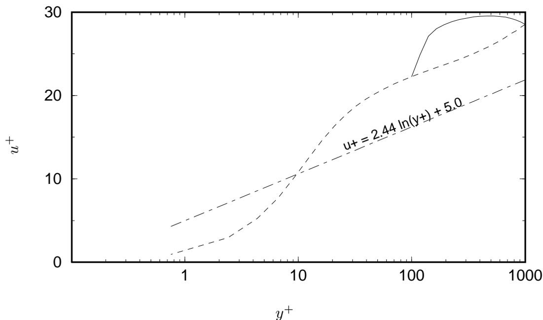
FIGURE 2. Mean velocity profile for the asymmetric computation.  $\gamma_u = \gamma_v = \gamma_w = 2$ . — : lower half, artificial boundary conditions; ---- : upper half, classical boundary conditions. Non-dimensionalization is based on the mean friction velocity.
