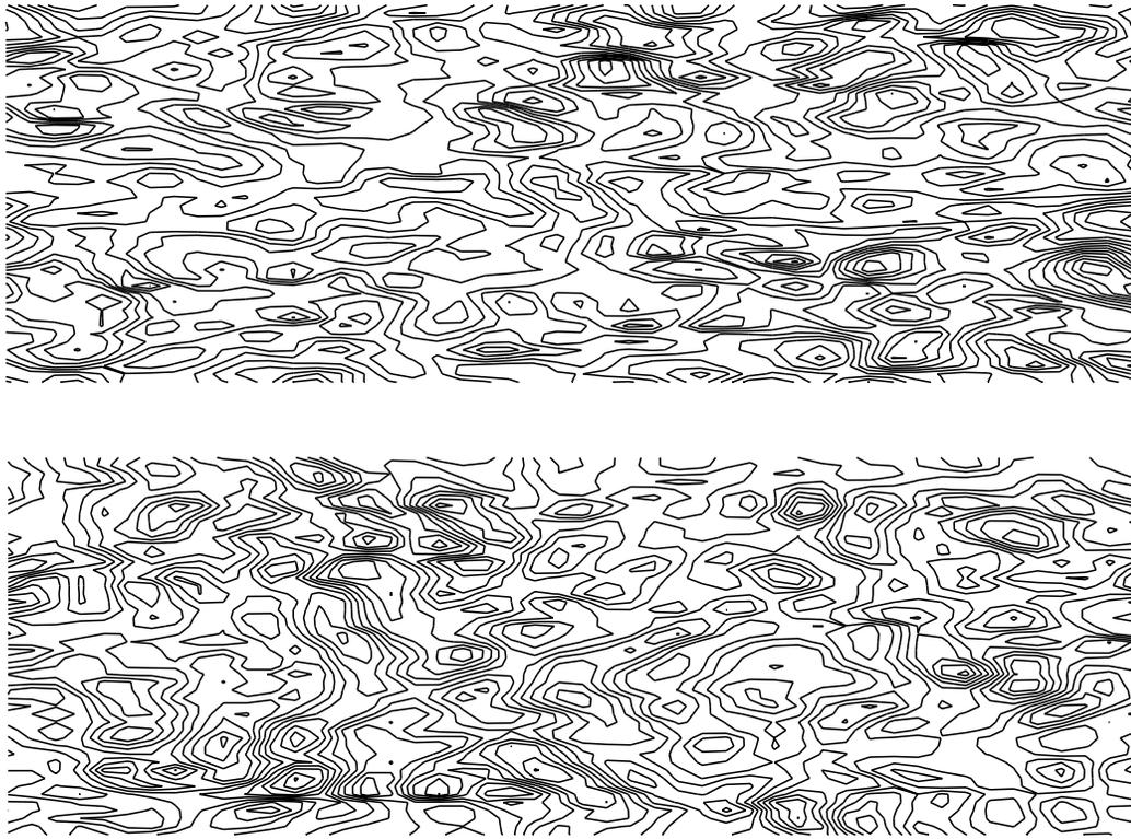
FIGURE 7. Iso-lines of  $v$ -velocity in the plane  $y = 0.8h$  (top) and  $y = -0.8h$  (bottom).  $\gamma$ 's computed dynamically. Flow is from left to right.
