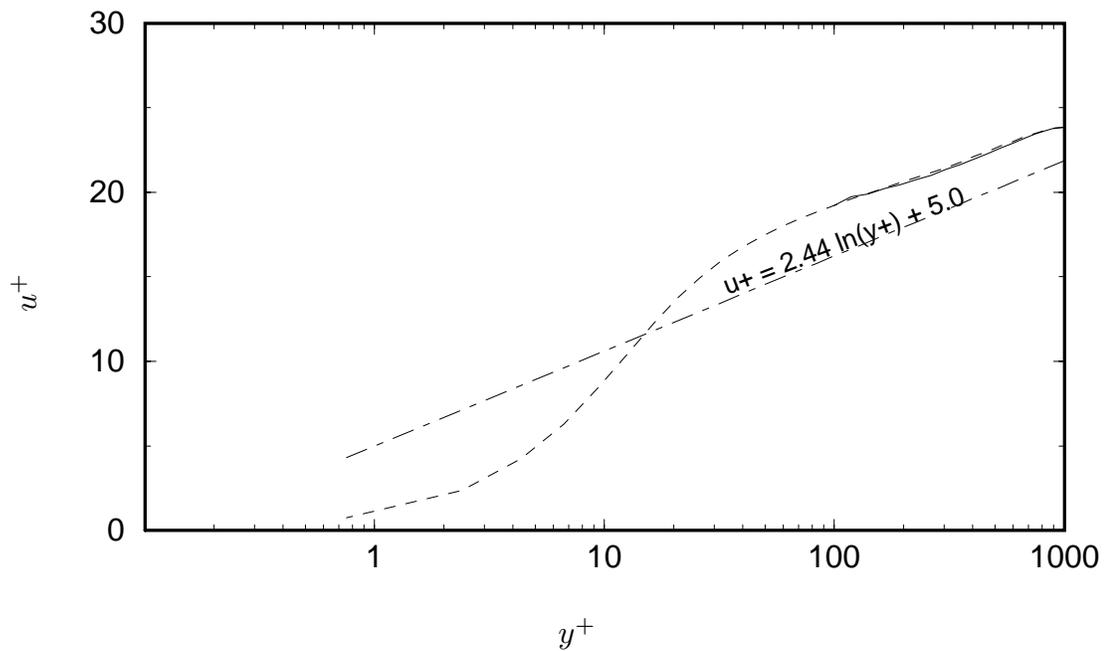
FIGURE 4. Mean velocity profile for the asymmetric computation.  $\gamma$ 's computed dynamically. — : lower half, artificial boundary conditions; ---- : upper half, classical boundary conditions.
