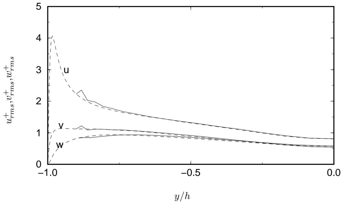
FIGURE 6. Turbulence intensities for the asymmetric computation.  $\gamma$ 's computed dynamically. — : lower half, artificial boundary conditions; ---- : upper half, classical boundary conditions.
