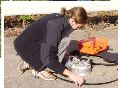
Flux accumulation chamber
