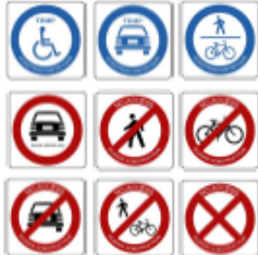
Detour and No-Access Signs *Coordinate the location of detour signs with the Project Management and Campus Circulation. *Provide detour sign locations and radius on Construction Project Site Plan. Detour Sign Template
