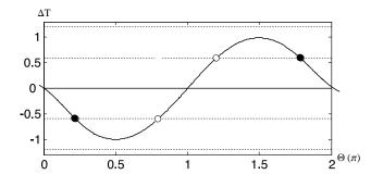
The Kuramoto model's sinusoidal phase-coupling corresponds to a PRC that is a flipped sinusoid. To obtain the Kuramoto model's coupling strength, *K*, we must multiply the PRC's maximum advance/delay,  $\Delta T_{max}$ , by the network's total spike rate.
