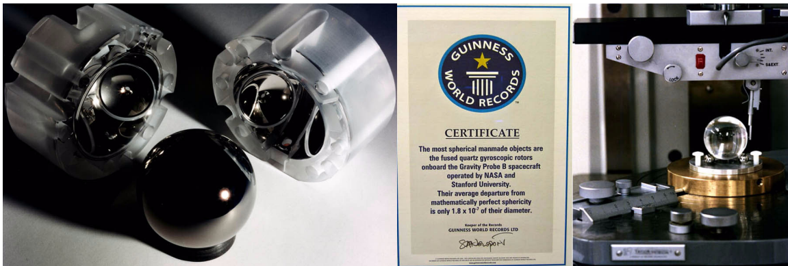
Figure 1-4. A GP-B niobium-coated gyro rotor and housing (left), the Guinness Database record for roundness (center), and measuring the sphericity of a gyro rotor (right)
