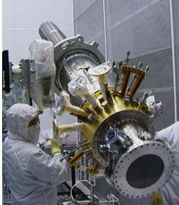
Figure 2-12. Final assembly of the Probe
