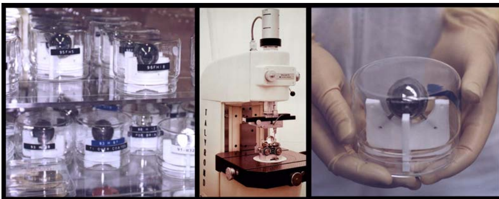
Figure 6-6. Gyroscope rotor development and precision sphericity measurement.
