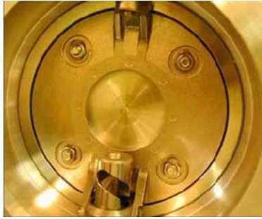
Figure 13-6. A six-inch Vatterfly leakage exhaust valve at the top of the dewar
