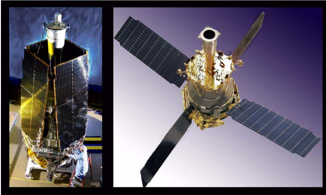
Figure 3-19. Checking the GP-B solar arrays on the spacecraft at Lockheed Martin & solar arrays deployed on a scale model of the spacecraft
