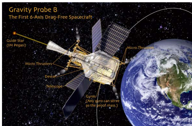
Figure 3-22. GP-B—The first spacecraft with 6 degrees of freedom in position and attitude control
