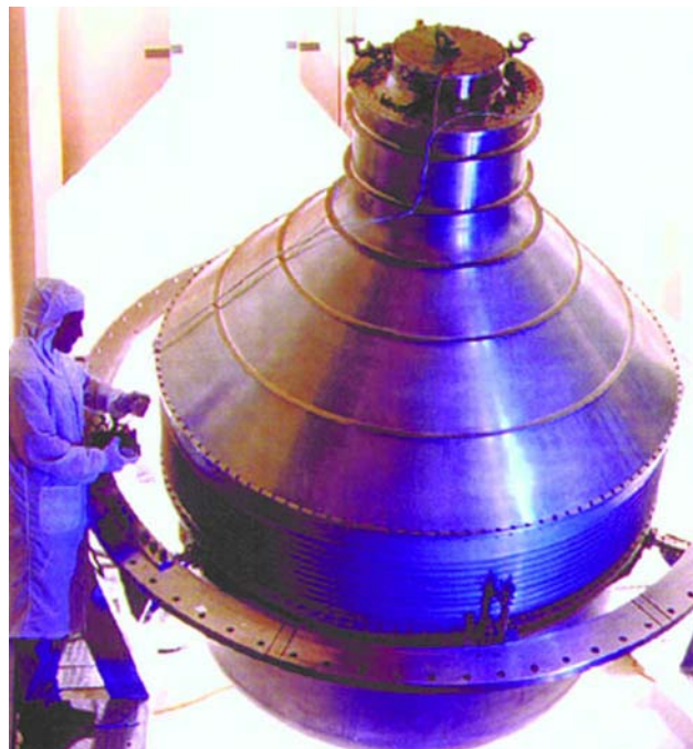
Figure 3-4. The GP-B dewar—one of the largest and most sophisticated dewars ever flown
