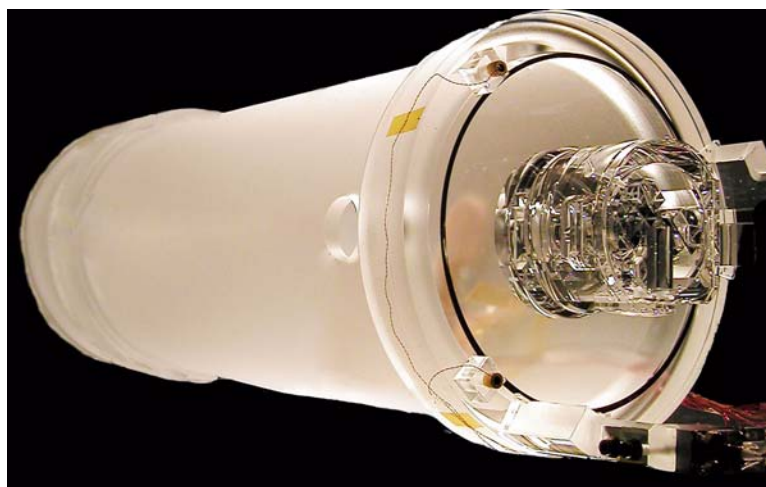
Figure 3-7. A pre-flight prototype of the Cassegrain telescope on-board the GP-B spacecraft
