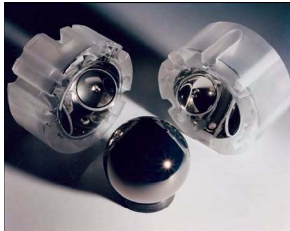
Figure 9-7. Photograph of rotor and housing. Suspension electrodes and spin-up channel are clearly seen.
