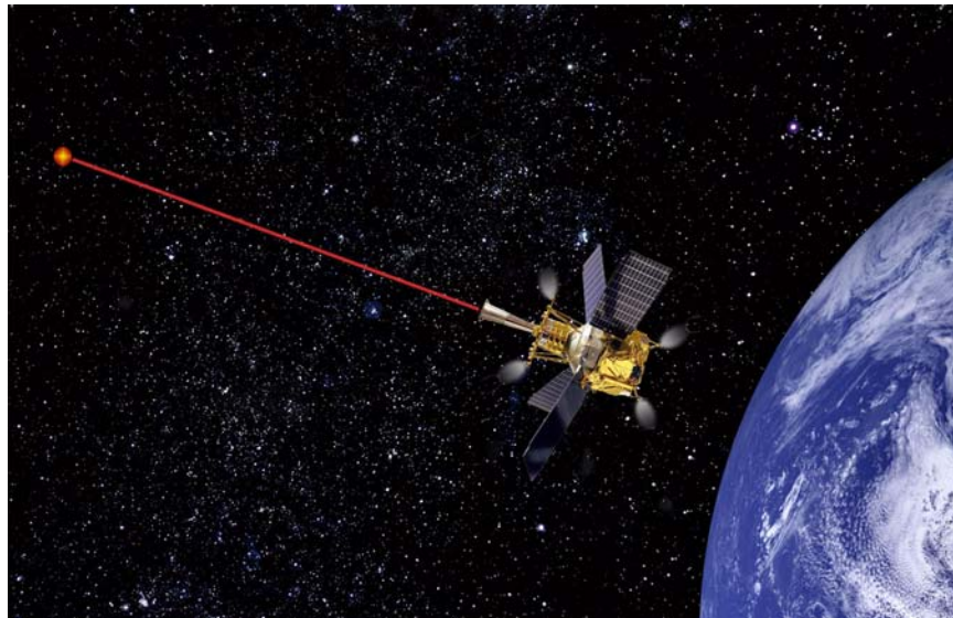
Figure 3-8. Tracking the guide star, IM Pegasi, with the GP-B telescope
