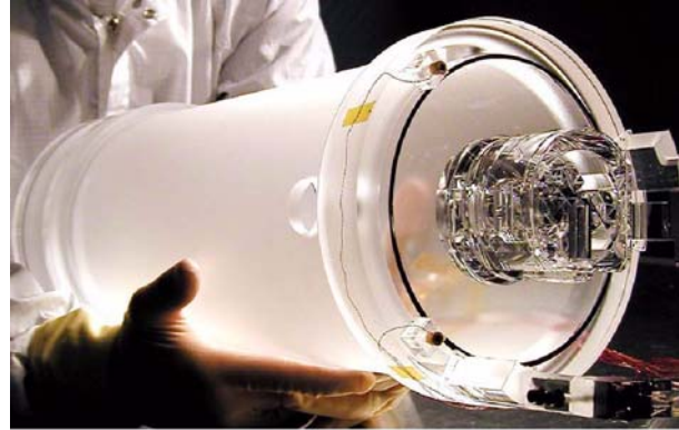
Side view of the pre-flight prototype Gp-B telescope. The actual flight version has clear sides.
