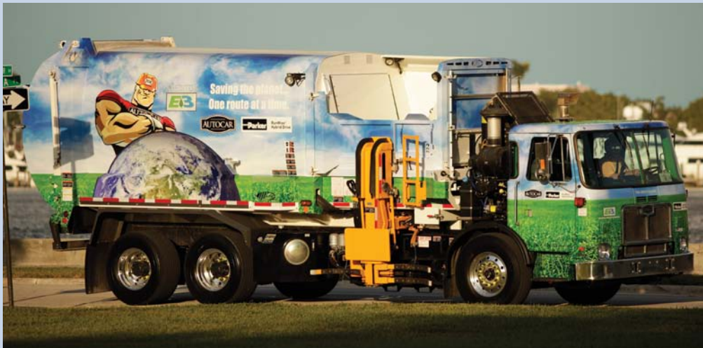
These fuel-efficient hydraulic hybrid refuse haulers now operate throughout Miami.
