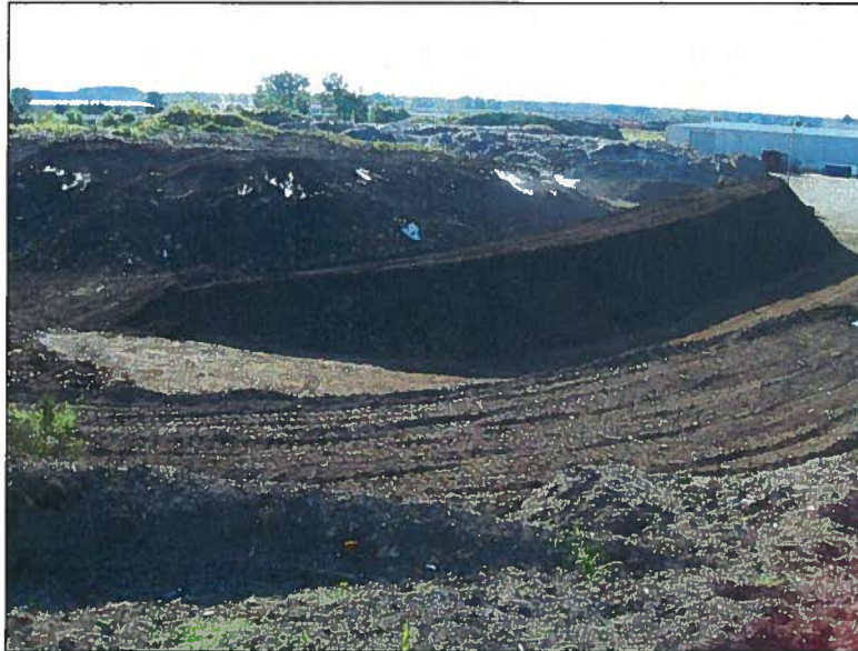
Photo 1. VIM Recycling, Inc., Elkhart operations Description: Engineered windrow of fines (< 4") on west side of C-Pile resulting from screening Date Taken: 9/18/09
