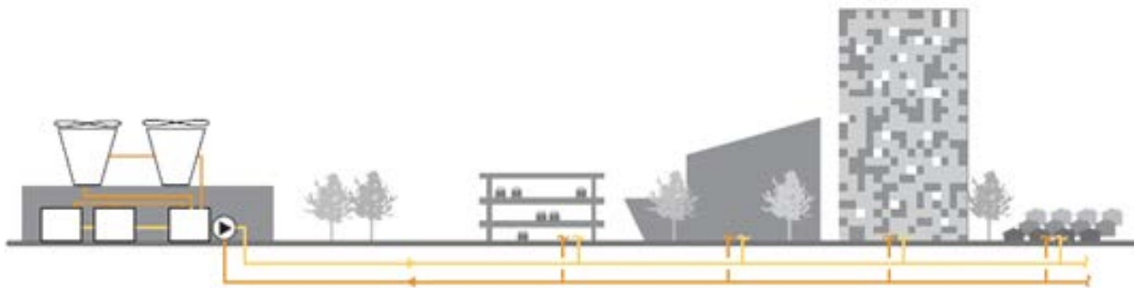
Figure B-3: This schematic diagram of a centralized condenser water system shows cooling towers in a central plant that delivers condenser water (yellow) to various connected buildings through a pipe network and returns water at a higher or lower temperature (dark orange), depending on whether it is being used for heating or cooling, to the plant.
