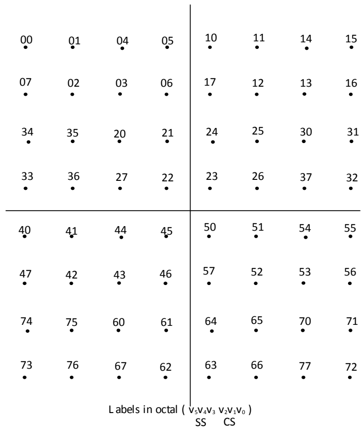
Figure 10.24: Constellation for 64QAM code example with 4.57dB gain.
