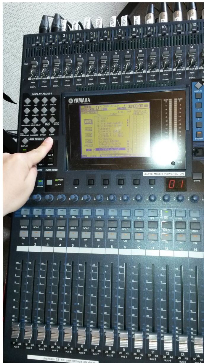
Fig. 1: Location of SCENE button in DISPLAY ACCESS; LED screen showing Scene menu
