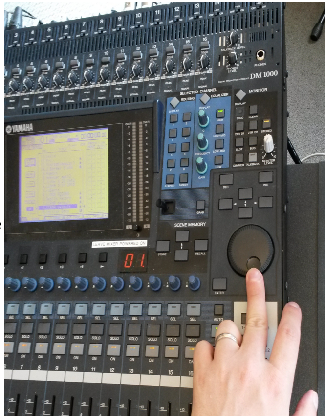
Fig. 2) Circular dial, cursor/arrow buttons (above) and ENTER button (below), SCENE MEMORY section (left), and red LED (farther left).
