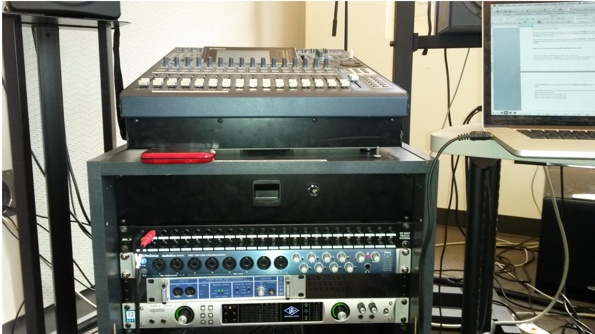
Fig. 3) Connection from 1/8 inch laptop jack to 1/4 inch patchbay input jacks 1 and 2
