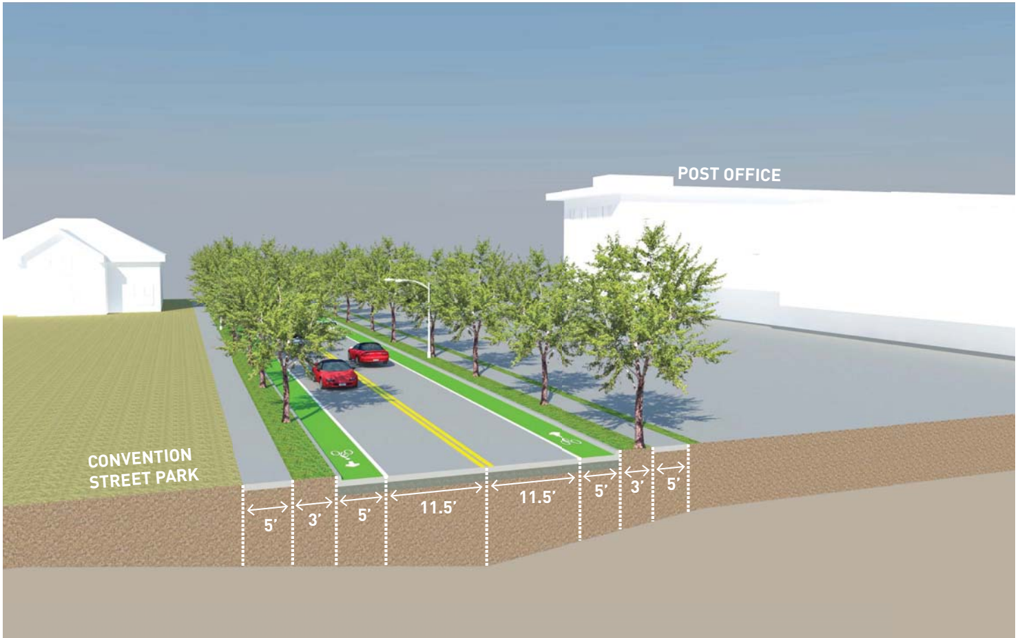
Figure 39: This image shows the design option for the street section through North 7 th Street.
